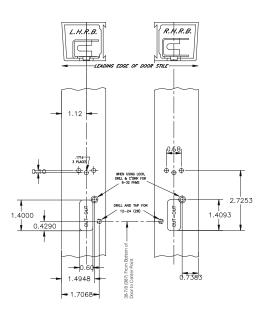
Install Rod & Case assembly into active stile. Secure with 2 ea. 8-32 x 1/4 soc. hd. cap screws.
