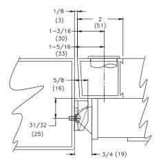
Locate mounting hole on inactive stile.
