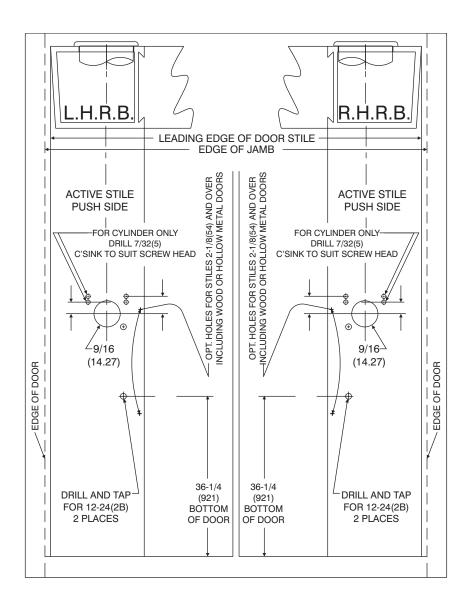
Locate centerline of cylinder on exterior of door and drill if required.
