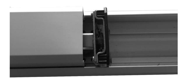
3. Lift the old end cap off the roller. Please pay attention to the way the end cap is installed over the roll, so you can install the new end cap in a similar fashion.
