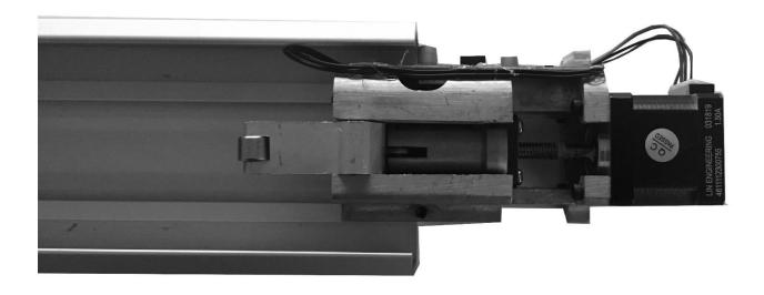
9. Slide the motor assembly into the bar, so it is within 1/8 of an inch from the end cap bracket when the push bar is depressed. Make sure that the push bar can move up and down freely with out anything coming in contact with the motor assembly.
